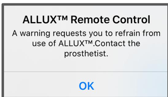
Because hydraulic control may be out of order, the control of ALLUX™ is stopped. Contact the prosthetist to have maintenance service.
