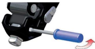
Fig. 20 Removing the Stance-Flexion Rubber
